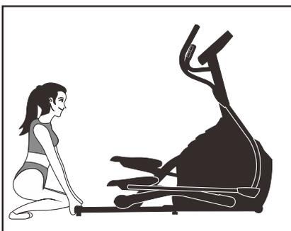
1. At the rear of the machine squat down and grasp the rear stabilizer bar.
