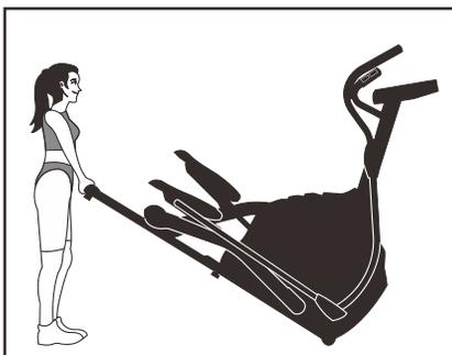
2. Lift the rear of the machine using your legs until the wheels in the front engage with the ground.
